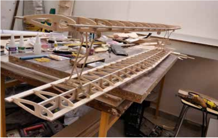
2. ABOVE – Basic wings construction. Struts are made of 3mm plywood. The ribs for connecting the struts are made of 2mm plywood. The central rib is made of 3mm plywood. The other ribs are made of 2mm balsa. The main spar of the wing is made of 5mm balsa.
