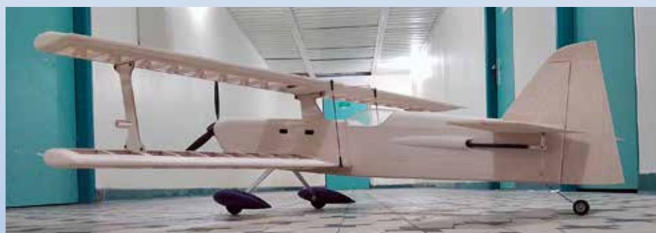
Finished frame of a biplane. Weight without engine was 760g
