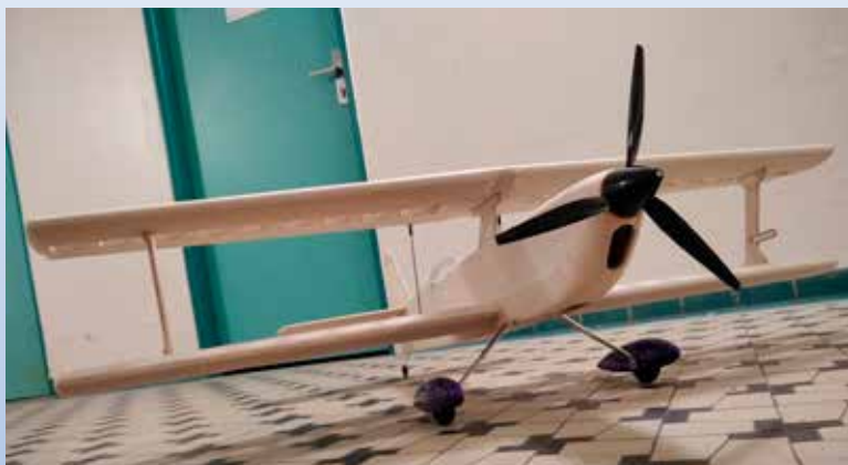
Plenty of air intake for cooling in the generous motor cowling.
