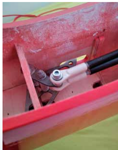
Two tie rods are attached to the Bellcrank. One is for the elevator and the other for the flaps.
