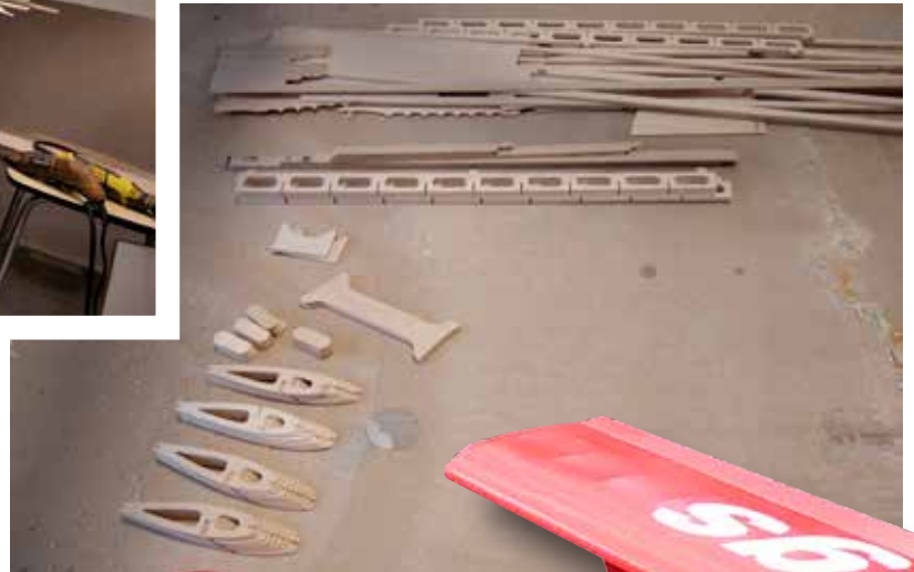
3. BELOW – Parts for the wing made on a CNC milling machine.
