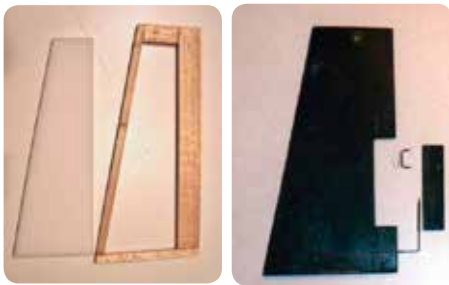
Two views, inside and then covered, of the stabilizer construction.
