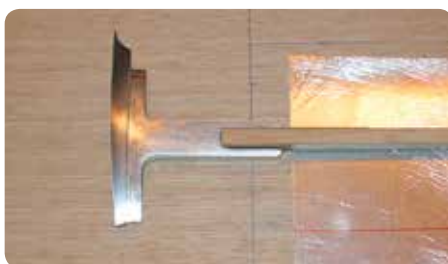
Detail of the spar and bellcrank holder. Note the sanded surface of wing sheet.
