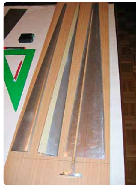
Finished wing, folded at 30° plus the spar with T-shaped bellcrank holder.
