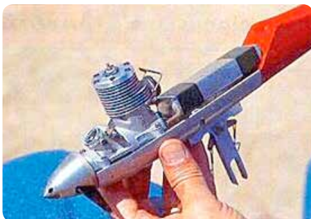
The tank is easily accessible when the cowl is removed.
