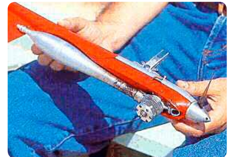
Everything assembled apart from the top cowl and the wing.
