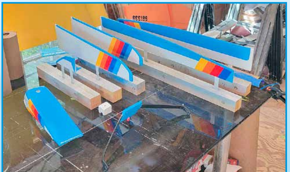
I use these stands all during the building process. The stands keep parts strait over time.
