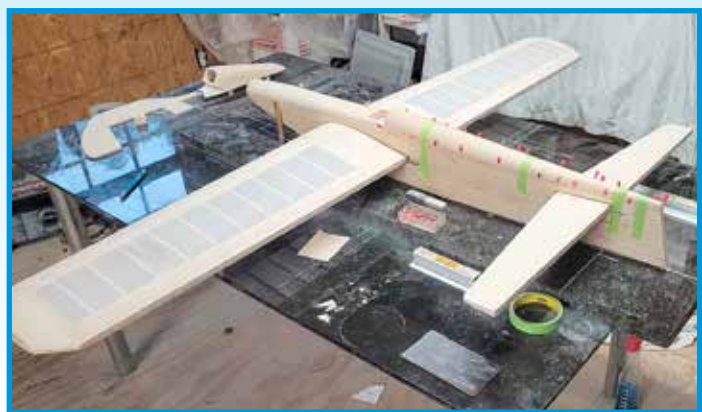
Molded top block being glued on after stabilizer installation.
