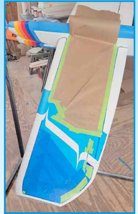
A combination of vinyl masks and hand masking were used to achieve the light blue trim on the wing.
