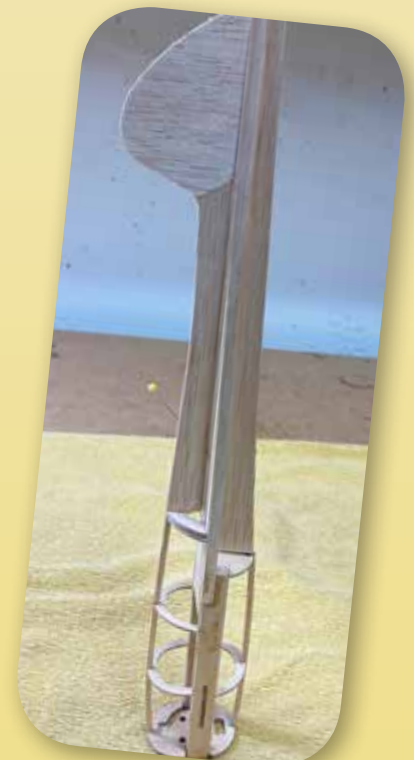
The skeleton of the fuselage glued together. It is always necessary to build light!
