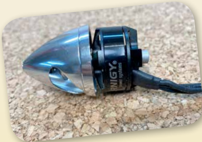
Engine and spinner. Note that spinner must stay within the dimensions specified in the rules for class 1.
